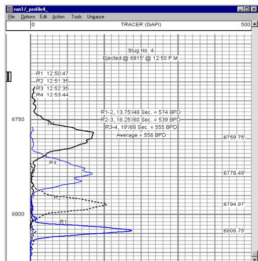
A no-flow shot is ejected between the bottom perforation and LTD. It is monitored in the same manner as the other velocity measurements. The primary objective is to determine if there is any fluid movement from below LTD in the casing. This is essential information. If the temperature surveys indicate fluid movement from below LTD, the no-flow shot is the only means to prove whether the movement is inside or outside the casing.
