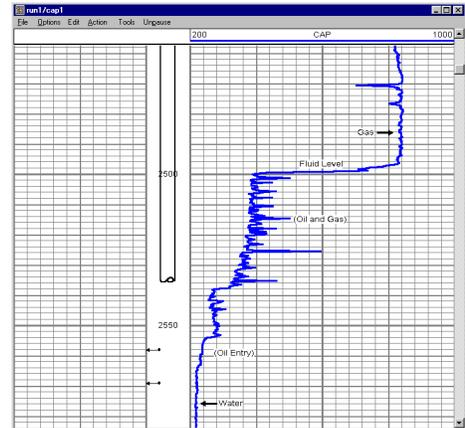
The next step is to run the radioactive tracer survey. The tracer will allow the determination of the direction and rate of fluid movement. There are the three basic components of the tracer: 100% shot, zone breakdown shots, and no-flow shots.
